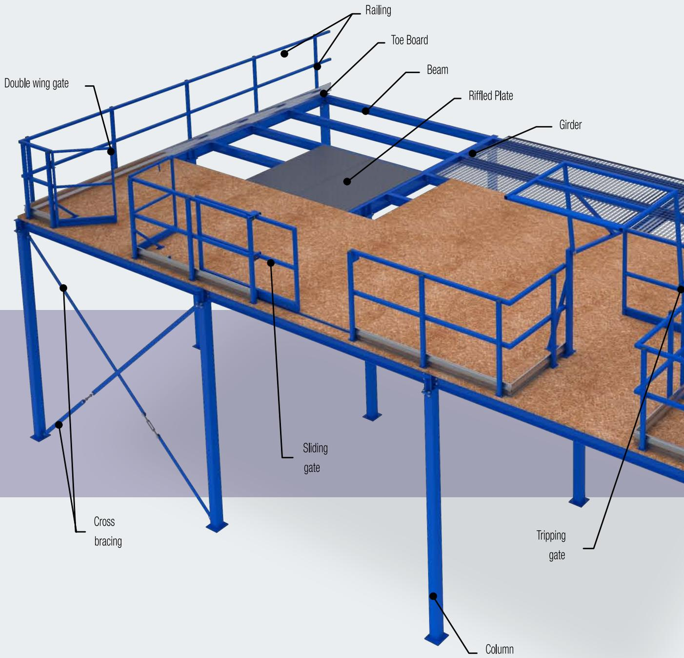
For usage of the platform it is necessary to have the minimum height of the room 4.5 m. In our solution the minimum walking height is 2.1 m. It is possible to equip the platform with different parts as lift, chute, netting, signs, lighting, etc.
